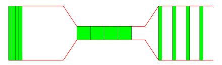
Figure: Measure the bottleneck using a burst of packets
